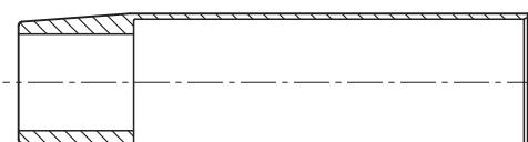
Mandrel P/N 20.0012.02 to assemble input shaft seal
