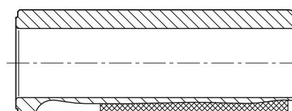
Mandrel P/N 20.1072.01 to assemble input shaft seal
