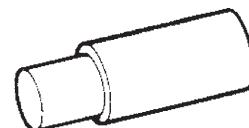
For assembling input shaft seal on the input spline side
