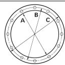
**Output Coupling Dimensions** Bolt Holes С В D Α Diameter (E) No. mm in mm in mm in mm in mm in 146 5.75 121 4.75 76.2 3.00 14.0 0.55 16.3 0.64
